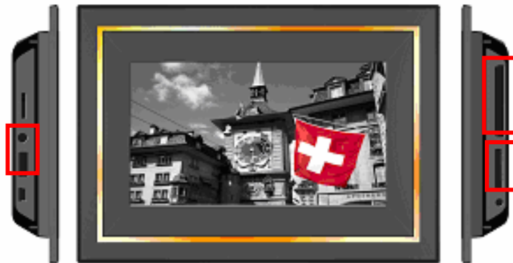
Figure 7: USB flash drive slot and memory card slots
